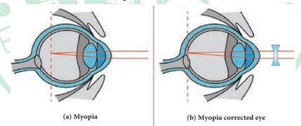
Let a person with myopia eye can see up to a distance x. Suppose that he wants to see all objects farther than this distance, i.e., up to infinity. Then the focal length of the required concave lens is f = -x. If the person can see up to a distance x and if he wishes to see up to a distance y, then, the focal length of the required concave lens is,
