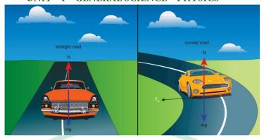
Suppose the road is horizontal then the normal force and gravitational force are exactly equal and opposite. The centripetal force is provided by the force of static friction Fs between the tyre and surface of the road which acts towards the centre of the circular track,
