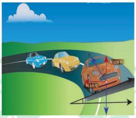
Let the surface of the road make angle  $\theta$  with horizontal surface. Then the normal force makes the same angle  $\theta$  with the vertical. When the car takes a turn, there are two forces acting on the car:
