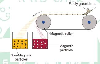
**Method:** The crushed ore is placed over a conveyer belt which rotates around two metal wheels, one of which is magnetic. The magnetic particles are attracted to the magnetic wheel and fall separately apart from the non-magnetic particles.
