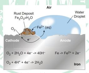
Rust is chemically known as hydrated ferric oxide (it is formulated as Fe2 O3. xH2 O). Rusting results in the formation of scaling reddish brown hydrated ferric oxide on the surface of iron and iron containing materials.
